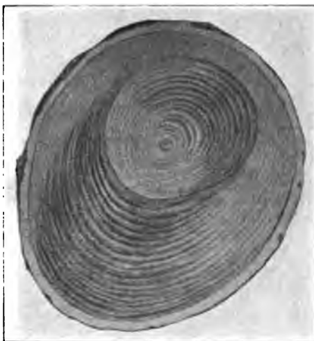
Fig. 117. Cross-section through a spruce branch. In the inner part of the wood disc the solid red wood is shown on the upper side of the branch but in the outer annual rings it is seen on the under side. (After R. Hartig.)
